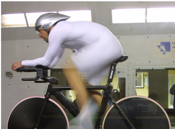
Drag measurement of track cyclists. Client : UK Sport
