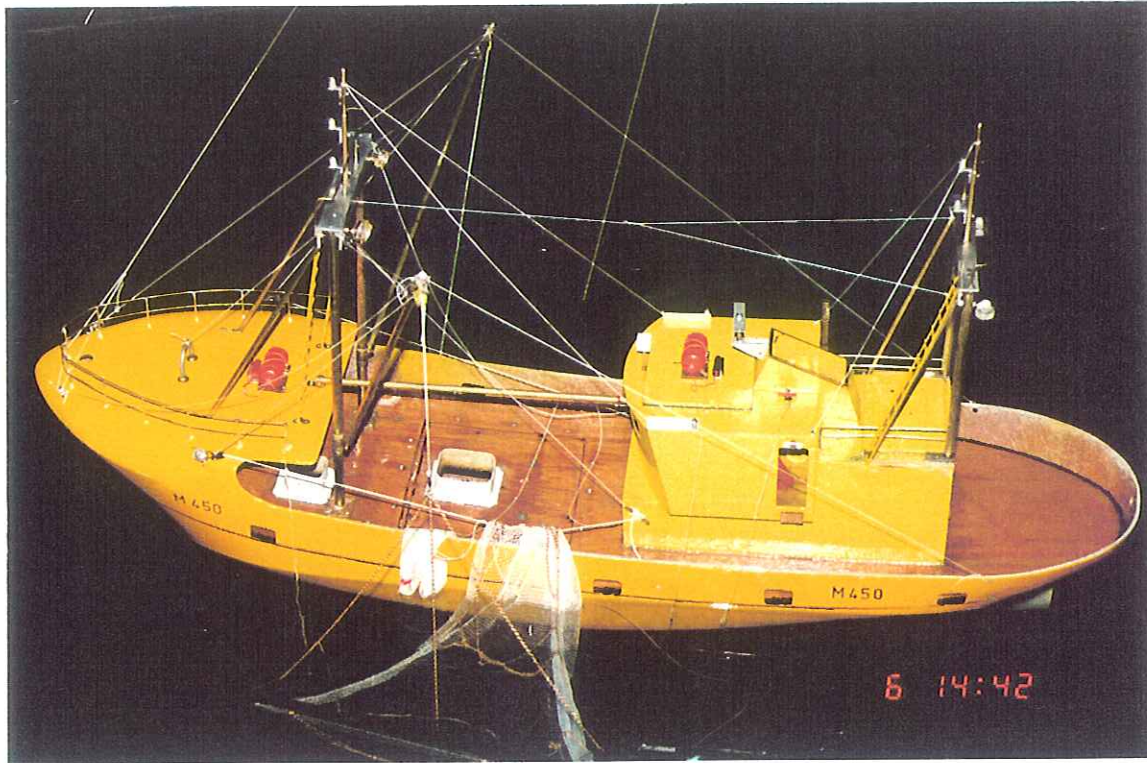
Figure 6. Beam trawler model with liferafts on wheelhouse and focsle. Preparing to haul on starboard trawl warp.
