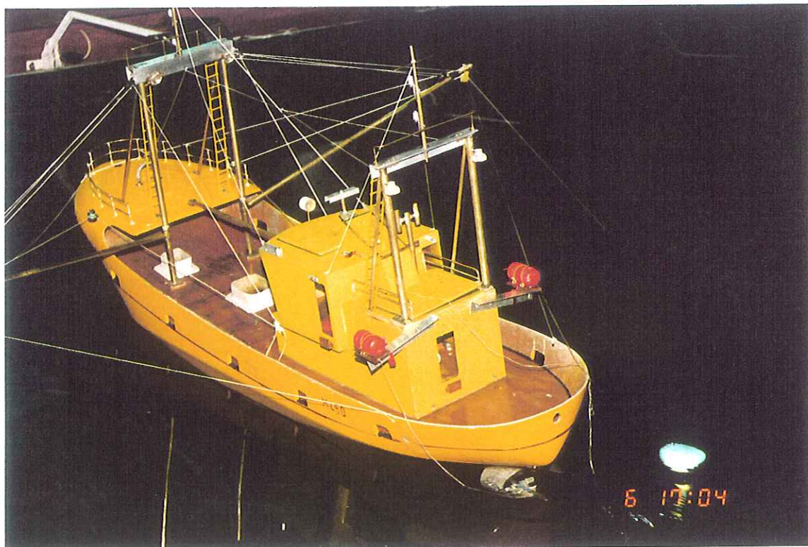
Figure 7. Beam trawler model with liferafts on brackets outboard of the galley. Preparing to haul on starboard trawl warp.
