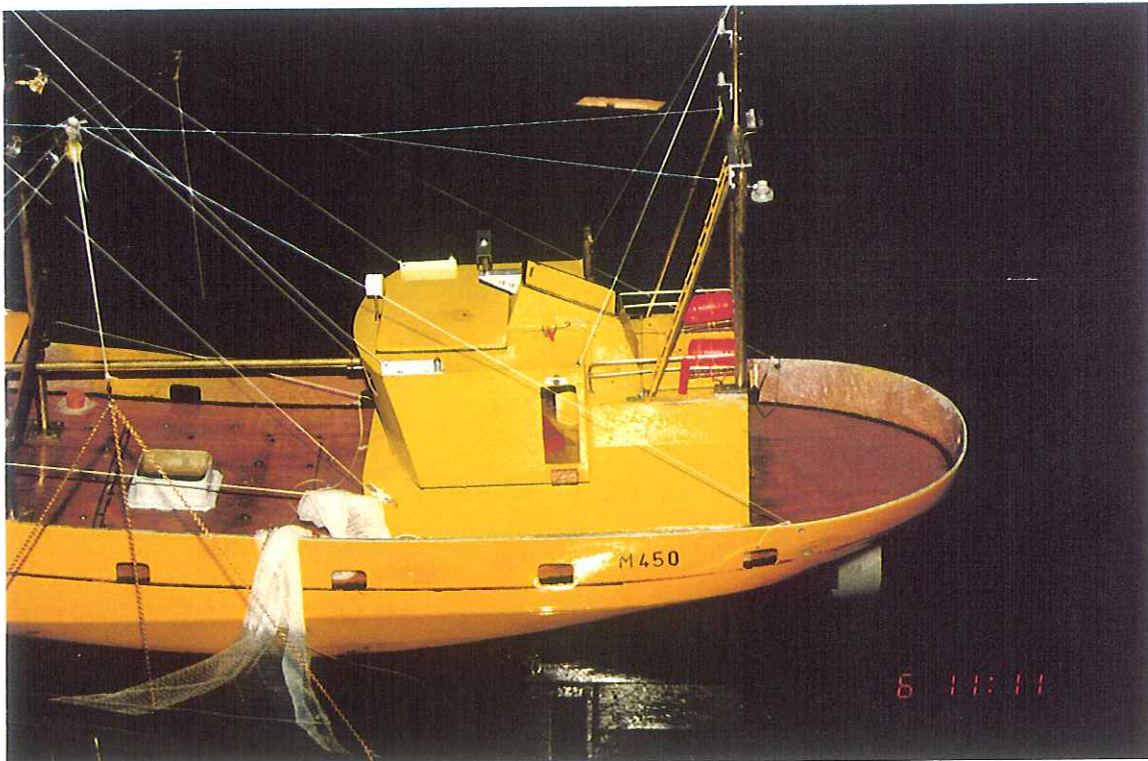
Figure 5. Beam trawler model with liferafts aft on the galley roof. Preparing to haul on starboard trawl warp.
