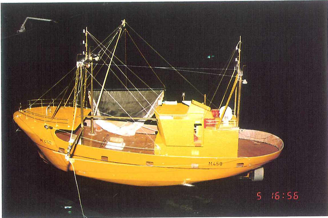
Figure 4. Beam trawler model with liferafts forward on the galley roof. Preparing to haul on port trawl warp.
