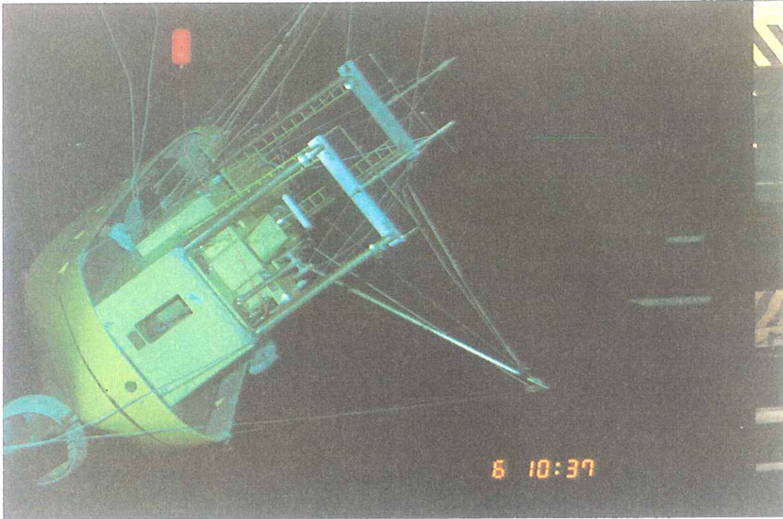
Figure 12. Beam trawler model on the tank bottom. Liferafts released from aft on galley roof. Starboard painter fouled on port trawl bridle.
