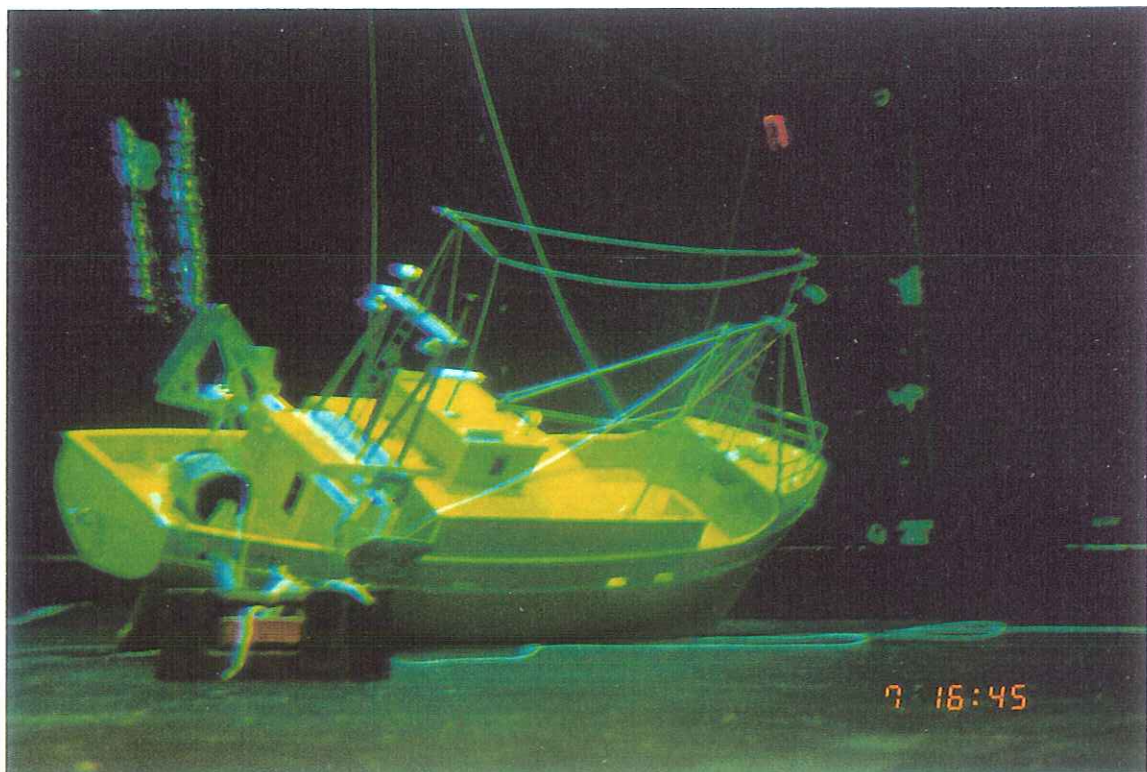
Figure 9. Westhaven model on the tank bottom. Liferaft released from shelter roof in front of wheelhouse, and passed through forward tripod mast.
