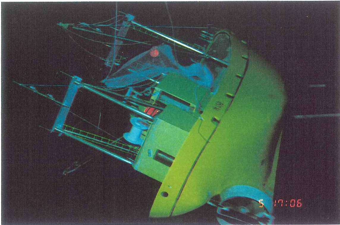
Figure 10. Beam trawler model on the tank bottom. Liferafts released from forward on galley roof. Port raft fouled in starboard trawl. Starboard canister jammed by railings.
