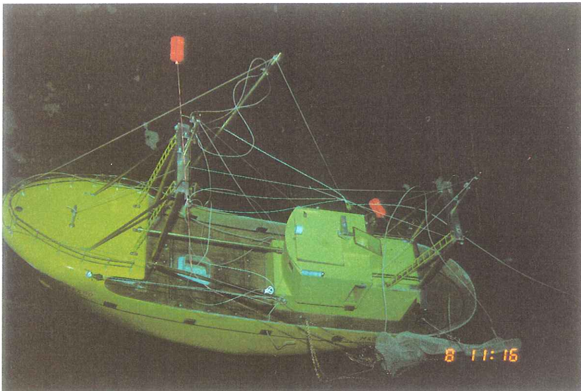
Figure 13. Beam trawler model on the tank bottom. Liferafts released from brackets outboard of galley. Starboard painter fouled on aft gantry. Port painter fouled on port boom, trawl warp and tickler chains.
