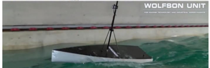
Un-restrained tests of an Open 60 in waves
